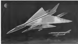
STAGED AIRCRAFT PROFILES made by Antonov Five is shown above in an actual conception. Dr. Fren believes that multi-stage or multi-wing air-lifting systems will be one conventional thin rocket-powered launchable aircraft over great ranges. Large first stage aircraft would accelerate the second vehicle with the gas load to supersonic speed and a high altitude. The second stage would use liquid air and the first fuelstage. Space between the stages would be optimized for best drag reduction at some speed below separation speed which would afford the greatest acceleration and altitude fuel load.
